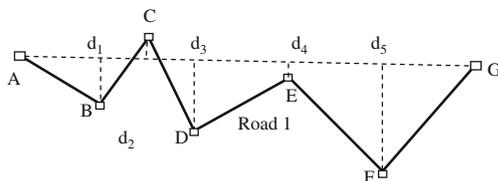
**Fig. 2** Principle of the distance-based method: the point  $F$  is selected, for it has the greatest distance to the line segment linking the two terminals of the edge
