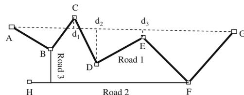
**Fig. 1** Demonstration of the intersection selection: for  $F$  and  $B$  are the terminals of Road 2 and Road 3, respectively, and have been selected,  $D$  is selected here, due to its greatest distance to  $AG$
