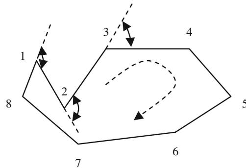
**Fig. 3** Deviation angle means an angle between the extension line and the other edge of the same joint vertex (the extension line is in anticlockwise of the polygon). The deviation angles of vertices 1, 2, and 3 are shown
