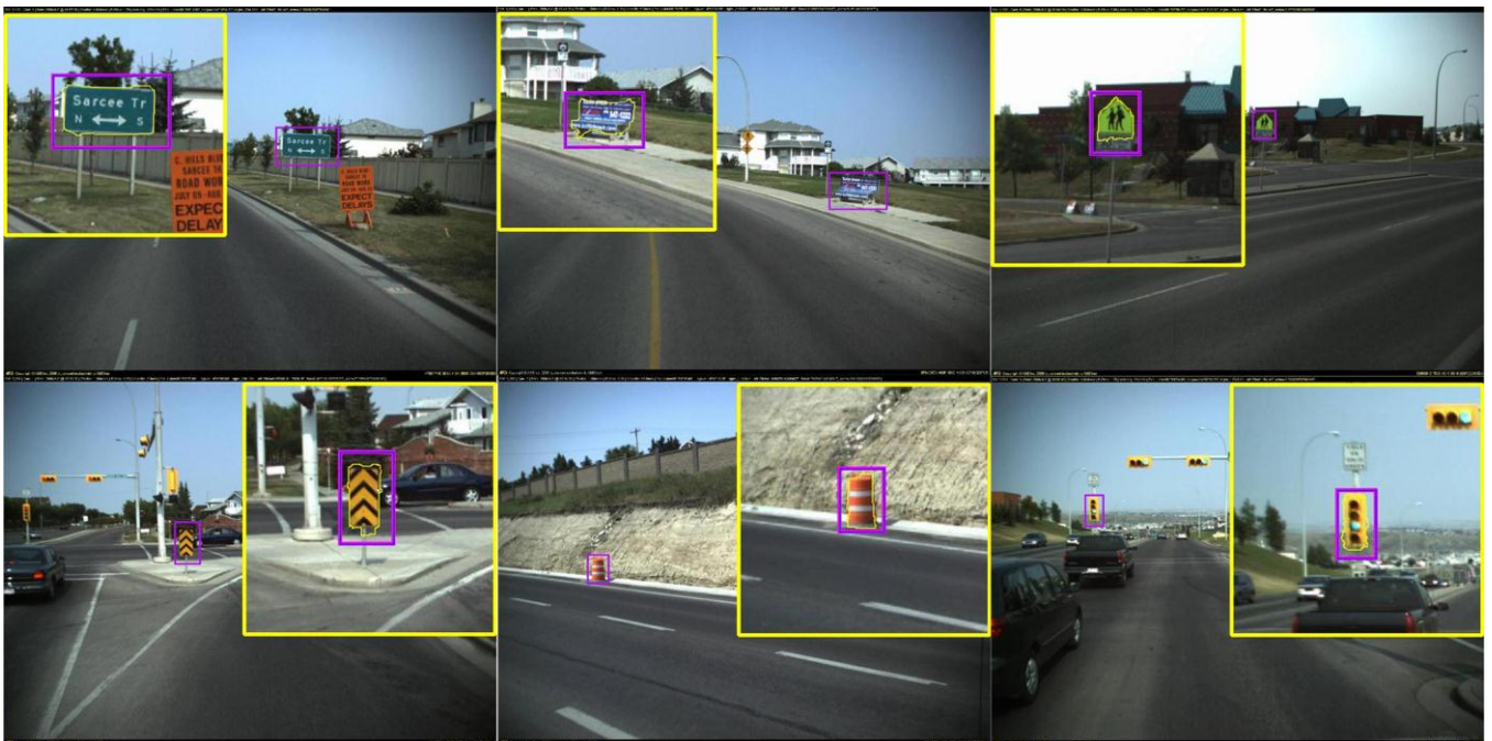
Figure 6. GIS OOI extraction for DMI sequences. The localization bounding boxes of the OOIs are shown in magenta and the contours are shown in yellow.
