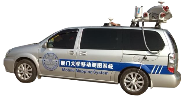
Figure 4. RIEGL VMX-450 mobile LiDAR system.
