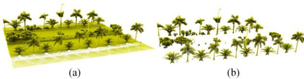
Figure 1. (a) Raw point cloud, and (b) off-ground points.
