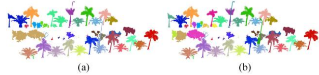
Figure 2. (a) Off-ground points clustering result, and (b) segmentation result of adjacent or overlapped objects.
