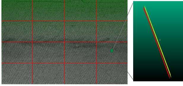
Fig. 4. Illustration of road block grid partition (left) strategy and two road surface profiles of a grid (right).
