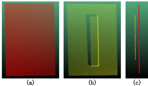
Fig. 9. Point cloud data for the simulated experiment: (a) the point cloud simulated as road surface before asphaltting, (b) the point cloud simulated as road surface after asphaltting and (c) two surface profiles detected using the proposed method.
