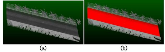
Fig. 2. Illustration of road surface segmentation result: (a) a raw MLS data and (b) the segmentation result of road and non-road points.
