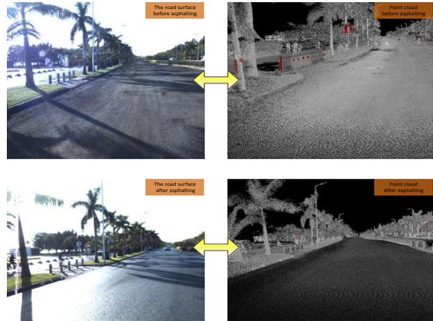
Fig. 8. Scene images and the corresponding point clouds acquired before (top) and after (bottom) asphaltting.
