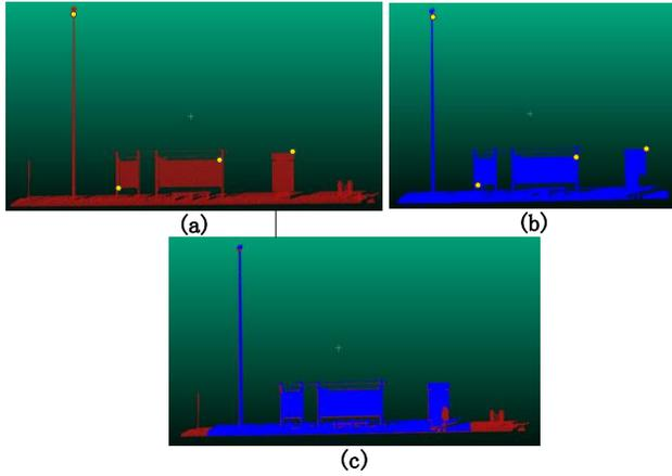
Fig. 1. Point cloud registration: (a) and (b) two point clouds with the same static targets (colored in yellow) coexisting in both of them, and (c) the registration result.
