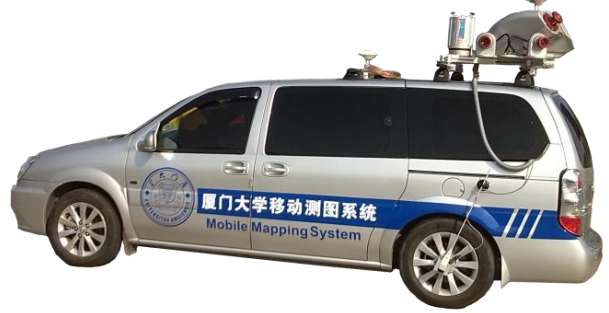
Fig. 2. RIEGL VMX-450 mobile LiDAR system and its components.
